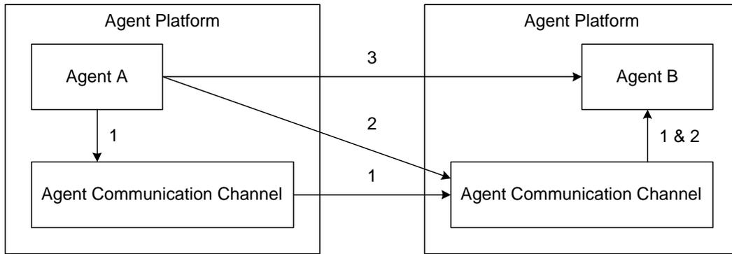
Figure 2: Three Methods of Communication between Agents on Different APs<sup>5</sup>
